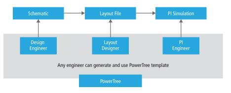
Figure 3: PowerTree technology enables the design engineer to have early visualization and define simulation criteria to ensure the layout designer's decap placement and PDN design meets target impedance requirements for each power rail on each component.
