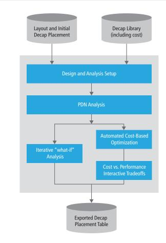
Figure 2: A Sigrity OptimizePI workflow for a post-layout optimization
