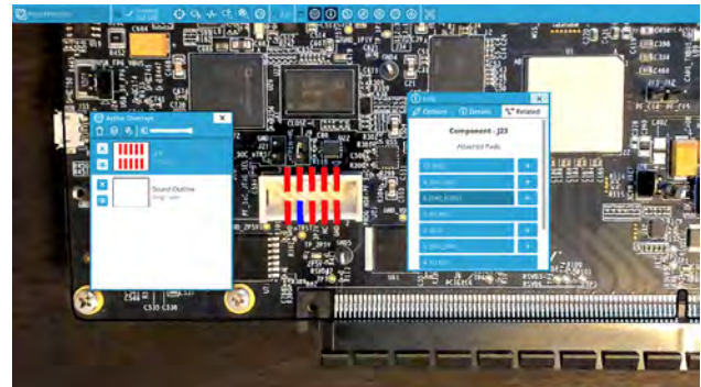
Figure 5: Active overlay of a component with related nets displayed in the information pane.
