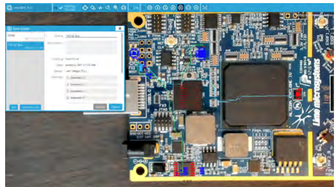
Figure 10: Color-by-Net allows users to differentiate between nets to minimize mistakes.
