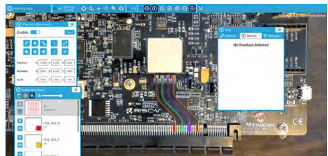
Figure 1: AR overlays active on a PCB
