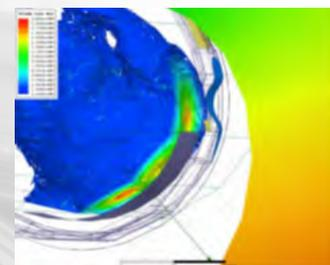
*Synapse Product Development used HFSS and the ANSYS human body model to evaluate the performance of various antenna designs by modeling the complete system, including the wireless device and antenna and their interactions with the human body.*
