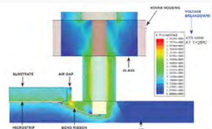
Raytheon engineers used ANSYS HFSS to compute the full electromagnetic field structure of a microwave antenna, and then coupled the HFSS model to ANSYS Mechanical to perform a transient thermal simulation.
