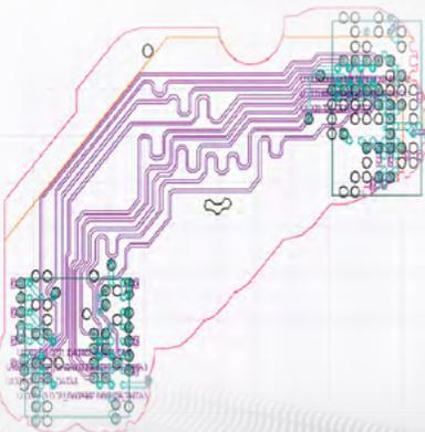
*Ooma saved 50 cents on each of hundreds of thousands of devices by using ANSYS HFSS and other ANSYS solutions to design a DDR3 subsystem that does not require a termination voltage regulator.*
