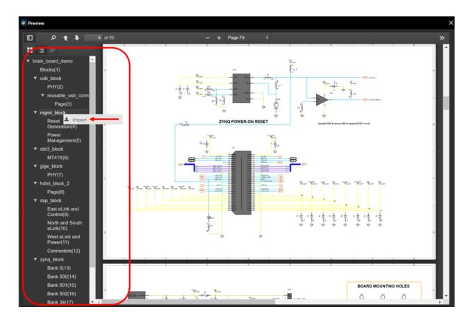
When a source design is committed and a change in it impacts a reused block, System Capture displays reuse update notifications for the blocks. You can view the differences to
