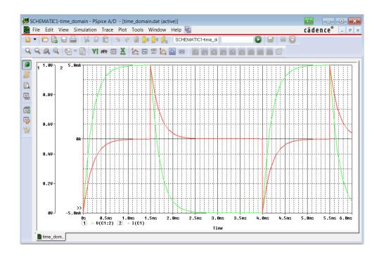
One of the simplest and most common variants of a timedependent process is e.g. the charging and discharging operation of a capacitor.
