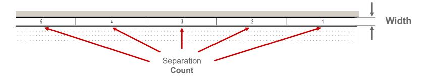
**Grid Reference** defines width of drawing frame as well as count of horizontal and vertical segments.
