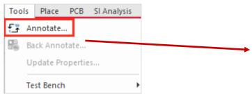
On previous page, we have assigned reference designators manually. During editing, Capture does not verify if duplicated reference designators exist (2 x U1, or 3 x R5). Verification happens during handover to PCB Editor.
