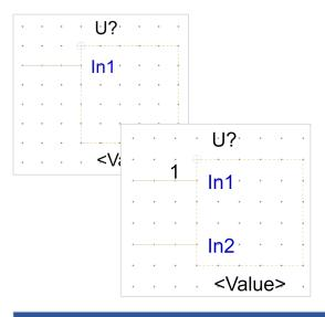
Additional pins can be placed by previous menu or by copy / paste (Ctrl C, Ctrl V).
