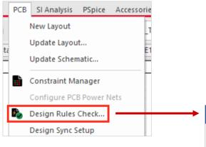
The DRC is able to identify one pin nets, nets without input or output. Pre condition is a correct defined library.
