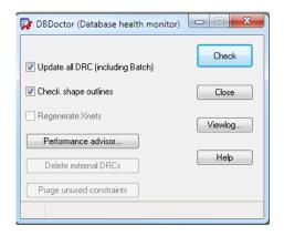
DBDoctor purges redundant vias and fixes any database errors found shown here in the viewlog:
