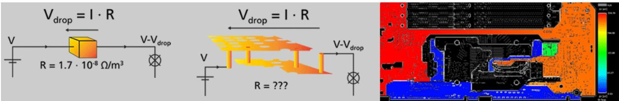
Power / ground paths should have low resistance. The goal is to ensure that minimum power is dissipated as heat in the system. Each voltage drop will generate heat and might cause thermal issues with some components close by.
