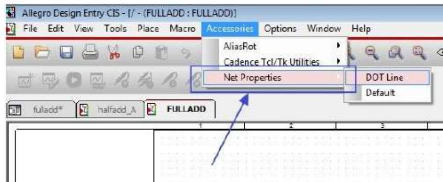
The menu contains popup for Line styles, namely **Dot Line** and **Default**. The user can select single or multiple nets on the schematic page and then choose one of the two options for assigning the desired net Line style. Following are the steps to do add the menu:
