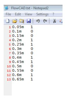
In this case we have first column for time (in milliseconds) and the second one for voltage (in this case volts).
