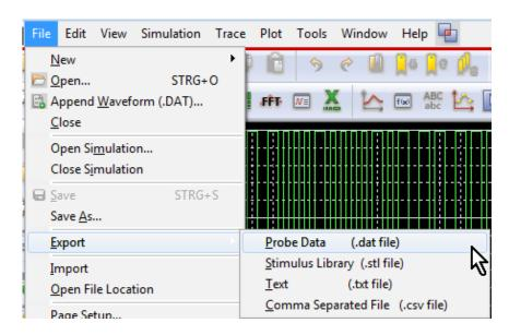
• From the plotted signals in PSpice Probe window, you can select the signals you want to export, then you click on **Ctrl+C** and then in a text file **Ctrl+V**.
