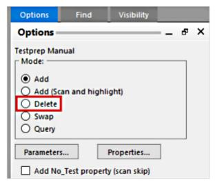
By selecting a testpoint you can delete a single testpoint. It's also possible to use area select to delete multiple testpoint at once.
