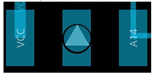
Allow test directly on trace: Auto generates a SMT pad to connect lines on external layers following all the restrictions defined.
