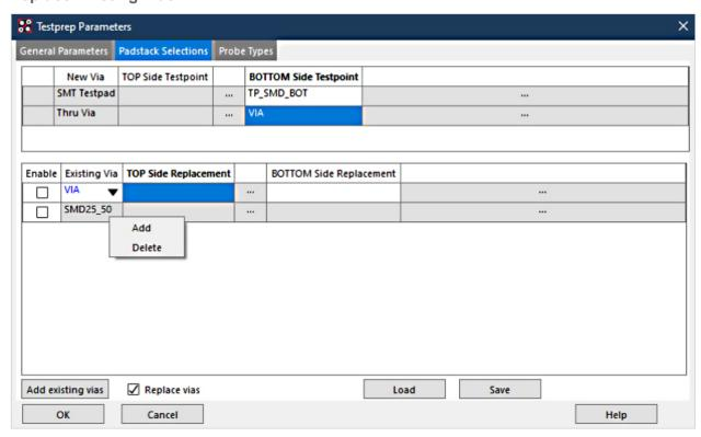
In the lower table you can define which existing testpoint via should be replaced. Initially, the table will be empty. The option **Load new existing vias** will populate the form with all vias used currently in the design.
