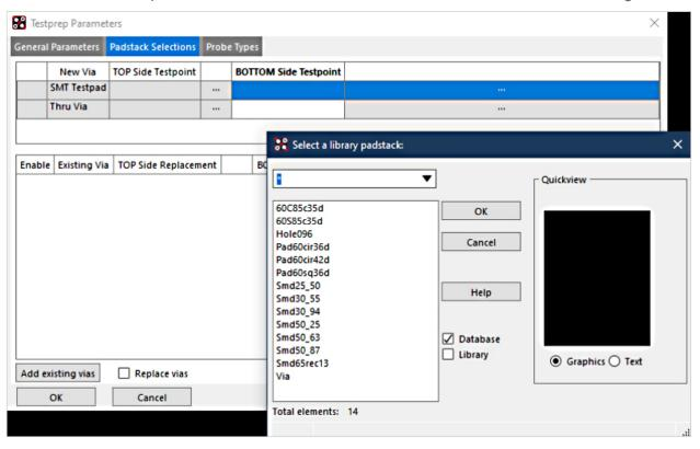
In the upper table it can be defined, which Pads or Vias are used when a new via or pad entity is being created as a testpoint.
