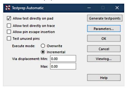
Allow test directly on pad: Specifies whether a pin or via can be selected as a test point:
