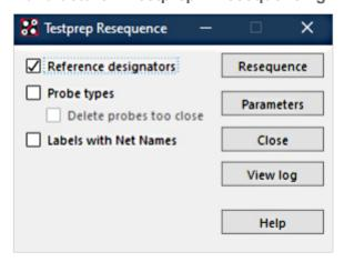
To test this function; Rename the refdes text of testpoints to ensure a visually sequential appearance, sorted by X / Y location from left to right and bottom to top on each side, starting with the TOP side first and then the BOTTOM side.
