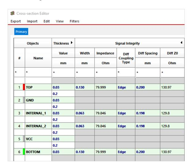
The Width and Diff Spacing values in the Cross Section Editor are not directly used as constraint values, as the calculator here is just a help for developing the cross section.
