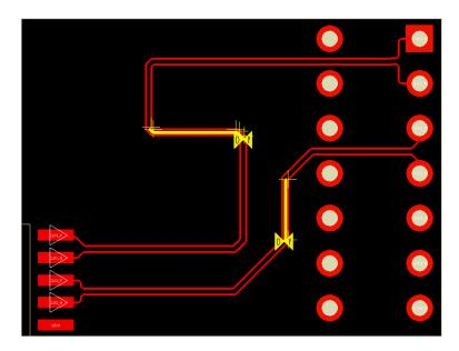
In the Constraint Manager the maximal allowed phase violation (tolerance) and the length, in which it has to be compensated, is defined. Again, actual routing and margin are displayed.
