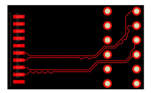
In the Constraint Manager the overall phase tolerance between the two members of the diff pair is defined and actual routed length difference and margin is displayed.
