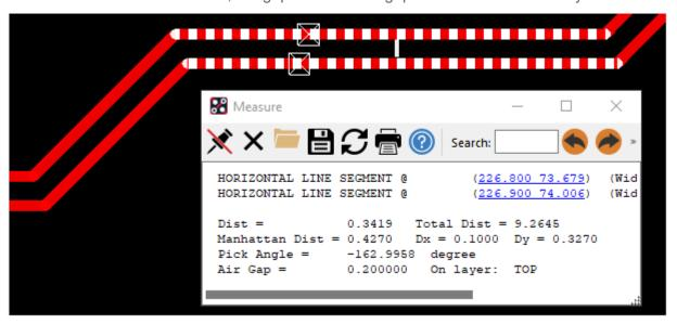
For line routed in 45 degrees or arcuated lines, the gap is slightly different due to calculation reasons. Here 0.20039 mm instead of 0.2 mm.
