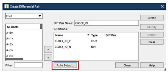
To filter for differential pairs, the + and - Filter can be used. It's also possible to set a prefix for the newly created diff pairs.
