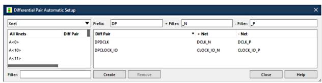
Auto Setup automatically lists all differential pairs and creates pair names. Select **Create**. Close log file, Differential Pairs Automatic Setup window and Create Differential Pair window. In Constraint Manager you will find all differential pairs:
