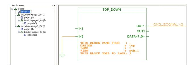
The Sample design has one page at the top level (TOP). The TOP page contains two identical blocks TOP\_DOWN (multiple instantiations) of one page schematic represented by page 2 and page 3. On each page 2 and page 3 additional blocks have been placed BLOCK1 (multiple instantiations). After cross-referencing, the design will consist of five pages, where Page 1 corresponds to the block TOP, pages 2 and 3 correspond to the block TOP\_DOWN, and pages 4 to 6 correspond to the block BLOCK1.
