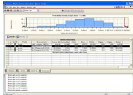
Figure 3: Monte Carlo predicts the behavior of a circuit statistically when part values are varied within their tolerance range.
